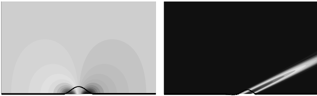
Fig. 4 Disturbance potential and mode shape for subsonic divergence (left) and supersonic flutter (right) corresponding to the parameters in Table 2.
